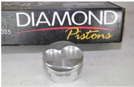
Diamond Pistons- Pins- Rings 540" Wedge- Original B-1 Heads 4.500 Bore- 4.250 Stroke 10cc Dome Top Gas Ports 7.100 Rod-.990 Pin.043-.043-3/16 Rings Price: $1,100
