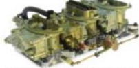
6 Pack OEM Holley Carbs *includes linkage, fuel line, vacuum secondaries, and 1 accelerator pump
